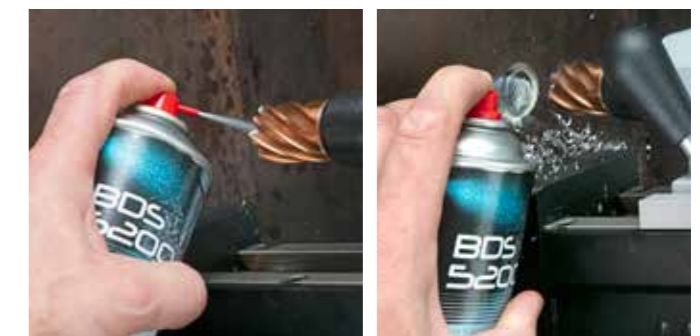
Step 1: Prior to drilling, spray the high-performance lubrication spray directly into the drill.
